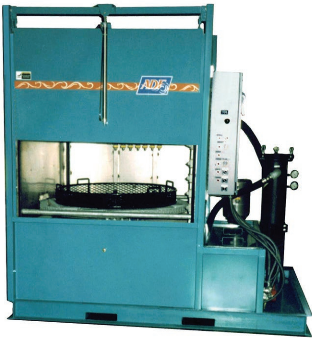
Shown with optional air doors. Filter and air blow off. Standard roller tables not shown.
