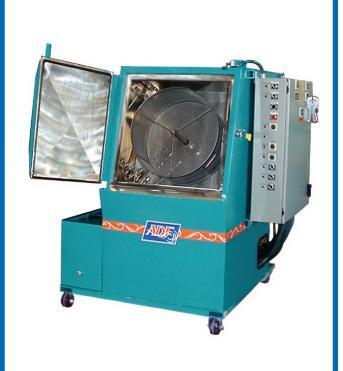
Rinse machine shown with optional recirculating rinse tank and hot compressed air blow off. Basket lid not shown.
