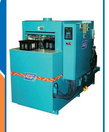
The Model 750 Rotary Basket Parts Washer is designed to clean parts that are best suited to being tumbled, rotated, immersed, and sprayed for proper cleaning. It offers the cleaning system needed for parts with blind holes, internal holes, cavities, threads, and those small parts that tend to nest preventing total cleaning. The hydraulic action of the fluid entering and evacuating the cavities offers excellent cleaning and rinsing.
